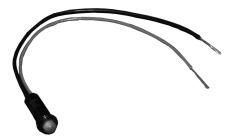
12-14 Volt LED Panel Lamp for .25" hole size. This series has typical LED (T1-3/4") Size. Lead wires are 6" long, stripped .380" on ends (red and black insulation indicates polarity).
